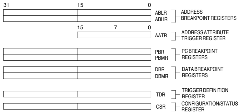
Figure 14-5. Debug Programming Model
